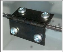
Proper Hinge installation:
