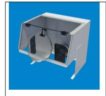
Insert Pre-assembled Rectangular Nozzle into the REAR WALL on the inside of the ClearView
