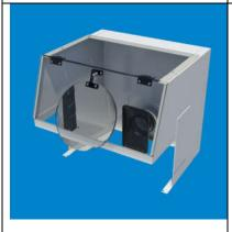
From parts kit, install plastic blank-off plate to the RIGHT side of ClearView Using (4) Longer screws
